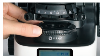
Turn the field diaphragm dial until the illumination range is circumscribed to the field of view.
